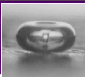
Cavitation near a solid surface can induce a microjet of liquid that streams through the bubble upon implosion.
