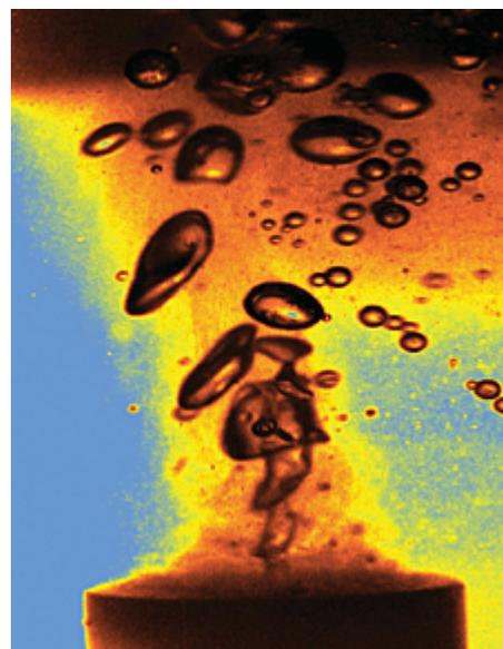
**SONOCHEMISTRY** A titanium rod vibrating at 20 kHz gives rise to a cloud of cavitating bubbles that emit flashes of light and house an array of chemical
