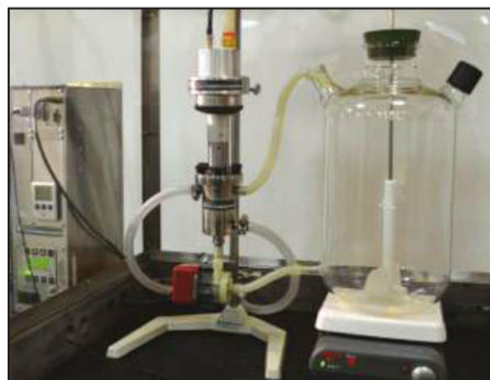
FIGURE 2. The BSP-1200 ultrasonic processor from Industrial Sonomechanics is designed for batch and flow-through processes and pilot-scale production. The processor outputs up to 1,200 W of acoustic power and operates at 20kHz
