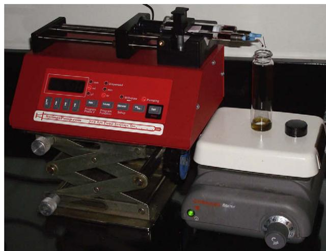
Figure 1. Photograph of slow addition setup.
