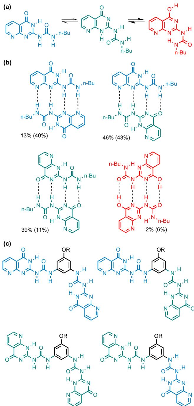
**Figure 5.** Self-association of ureidodeazapterin (DeAP) regardless of tautomerism. (a) Self-complementary protomeric forms of DeAP. Two non-complementary protomeric forms omitted. (b) Dimers of DeAP with percentage of each dimer in toluene- $d_6$  ( $\text{CDCl}_3$ ) as measured by  $^1\text{H}$  NMR.<sup>12</sup> (c) Four likely stereoisomers of Bis-DeAP after considering the multiple tautomeric forms of DeAP.
