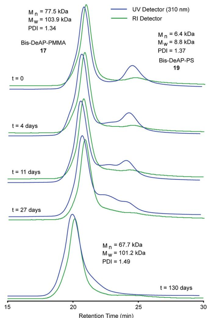
**Figure 10.** Bis-DeAP-PMMA, **17**, and Bis-DeAP-PS, **19**, mixed in toluene at room temperature. Aliquots analyzed by toluene SEC. Molecular weights determined from RI signal using conventional calibration with polystyrene standards.
