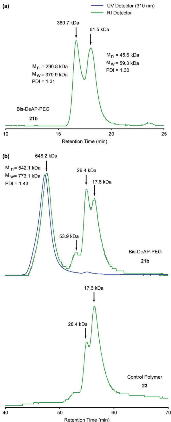
**Figure 15.** (a) SEC analysis of Bis-DeAP-20K-PEG **21b** in DMF. (b) SEC analysis of Bis-DeAP-20K-PEG **21b** and control polymer **23** in water. SEC samples prepared at approximately 7 mg/mL.
