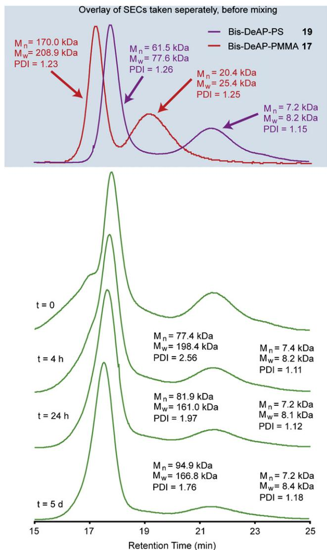
**Figure 12.** Relatively fast mixing of Bis-DeAP-PMMA **17** and Bis-DeAP-PS **19** in DMF at room temperature to generate a star copolymer through self-assembly. Molecular weights determined from DMF SEC (50 mM LiBr, 50 °C) using RI detection and conventional calibration with polystyrene standards.
