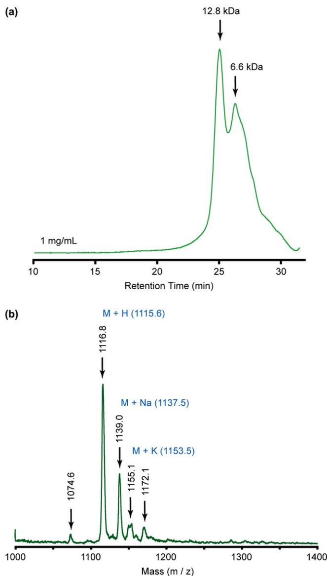
**Figure 6.** (a) THF SEC of Bis-DeAP-OH, **1**, using an RI detector. Molecular weights determined using conventional calibration with polystyrene standards. (b) MALDI mass spectrum of **1** using IAA as matrix.
