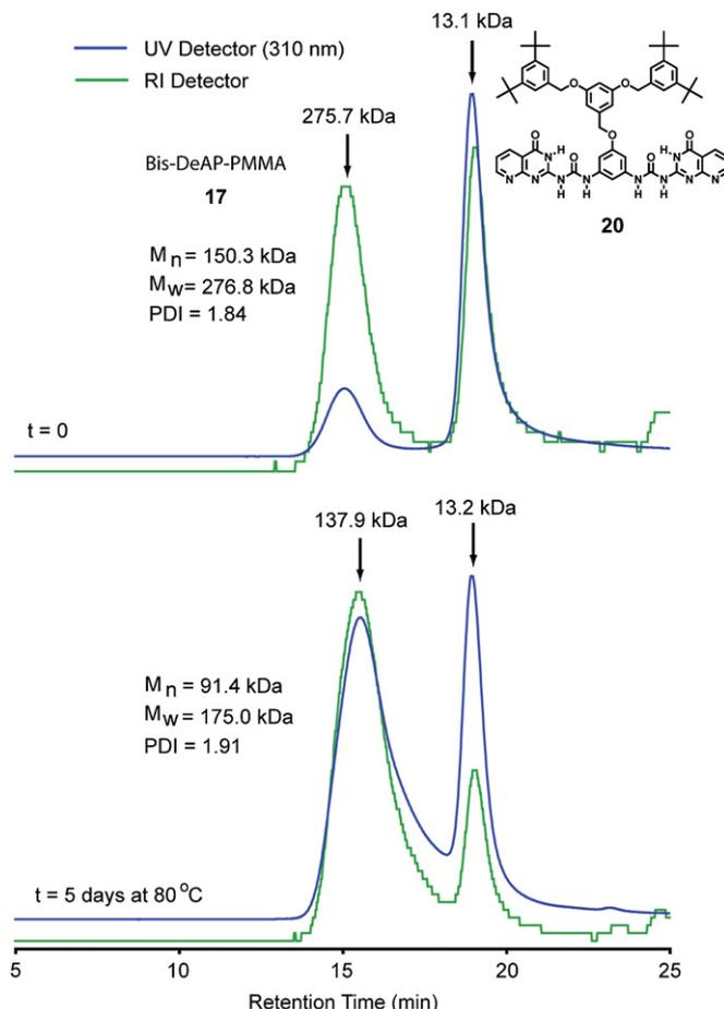
**Figure 11.** Bis-DeAP-PMMA, **17**, and Bis-DeAP, **20**, mixed in toluene at 80 °C. Aliquots analyzed by toluene SEC at room temperature. Molecular weights determined from RI signal using conventional calibration with polystyrene standards.
