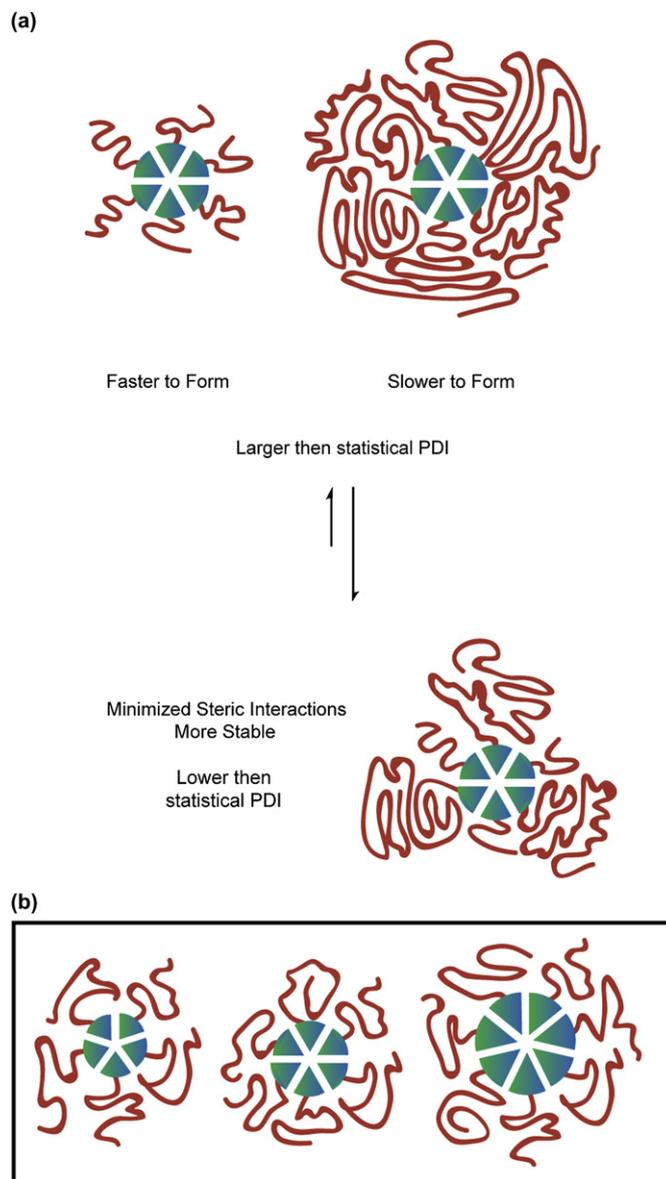
**Figure 13.** Schematic representation of possible explanations for larger than statistical PDI. (a) Initially the smaller polymeric material assembles first followed by the larger material leading to a kinetically controlled molecular weight distribution. Sterically the polymer coils should want to alternate between large and small leading to a thermodynamically controlled molecular weight distribution. (b) The original star polymer distribution contains multiple discrete aggregates.
