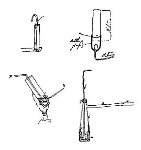
The evolution of Faraday's vessels for electrolysis of fused lead fluoride: 20 Jan. 1834 (top 1), 29 Jan. 1834 (top r), 10 Feb. 1834 (bottom 1), and 19 Feb. 1835 (bottom r) (31).
