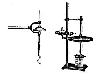
Turn-of-the-century laboratory stirrers. (Left): A stirrer with variable speed. (Right): A stirrer with the water motor attached.
