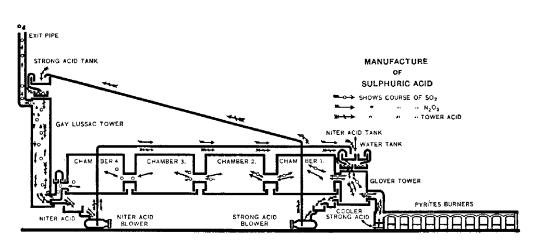
The lead chamber process for sulfuric acid as diagrammed in the 1909 edition of Thorp's Outlines of Industrial Chemistry.
