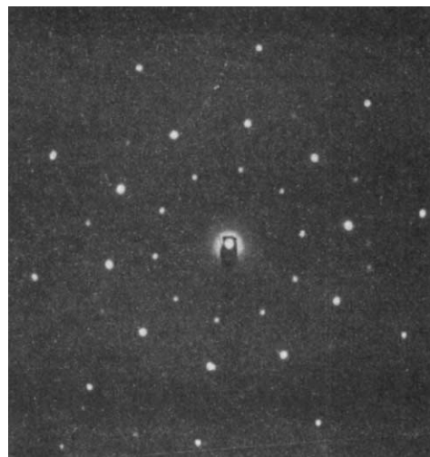
Fig. 1 Electron diffraction pattern from a \text{Ga}_{1.0}\text{Mg}_{1.8}\text{Zn}_{2.1} icosahedral crystal in a melt-spun ribbon.
