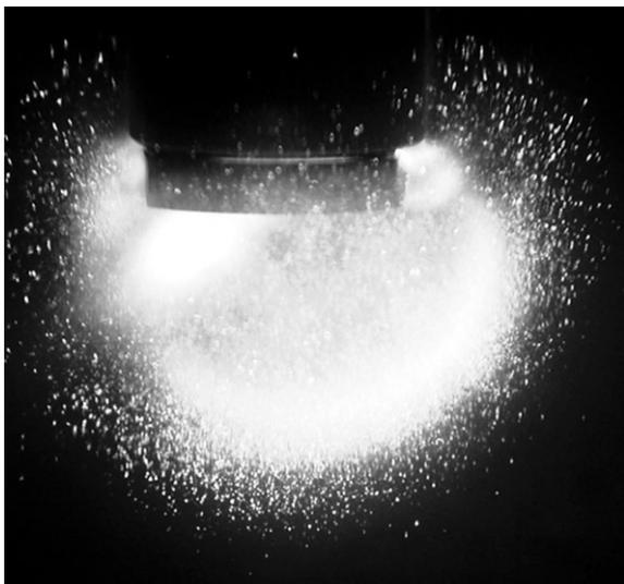
**Fig. 1.** MBSL. A photo of a MBSL cloud from an ultrasonic horn (1 cm diameter) in 95 wt.%  $\text{H}_2\text{SO}_4$  under Xe is shown.
